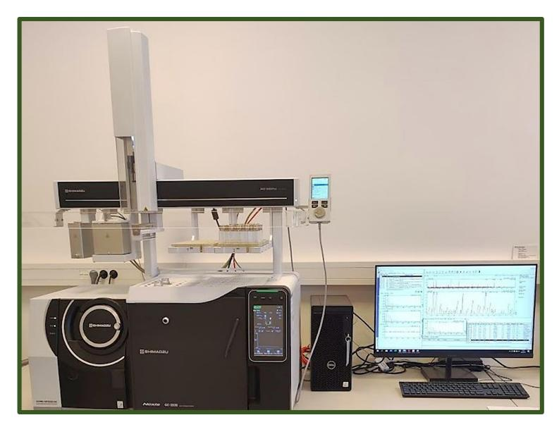
2. Volatiles were identified using HS-SPME-GC-MS
